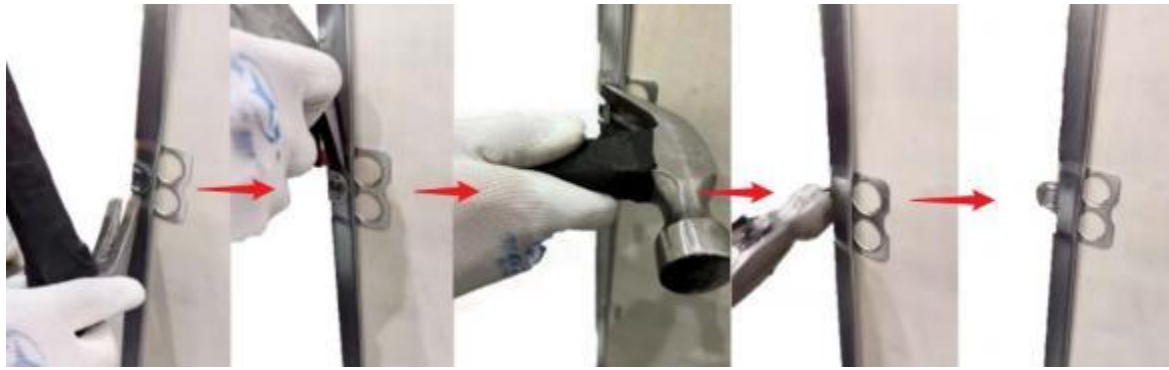
Fig. 4-2 Schematic Diagram of the Removal of the Wooden Box
